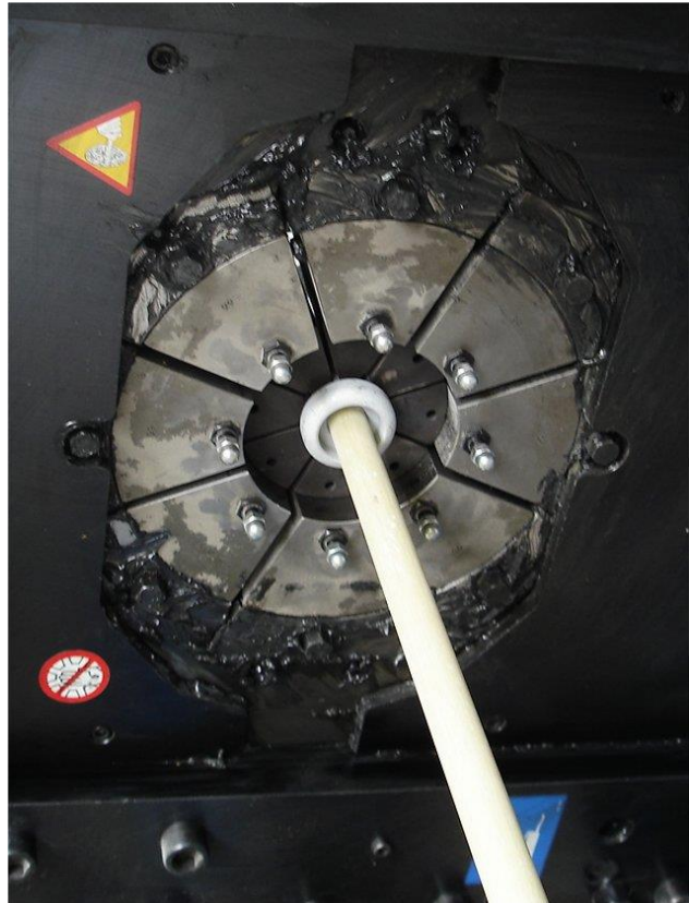
Fig. 7: Joining a fitting and a fiber glass rod by a crimping process
