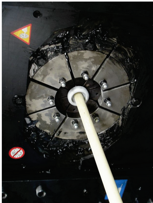
Figure 13: Joining a fitting and a fiber glass rod by a crimping process
