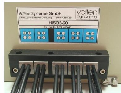
Figure 6-7 Front view on cable entry system (Ex i cables) and earth connection point
