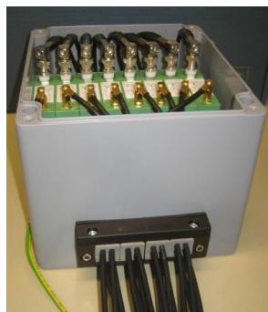
Figure 6-2 Front view on cable entry system
