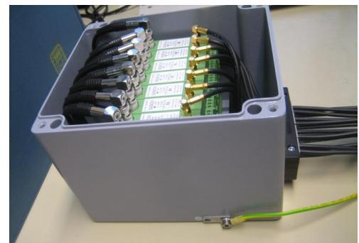
Figure 6-3 Side view on earth connection point
