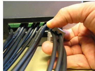
Figure 6-12 Clamp 4 cables into
