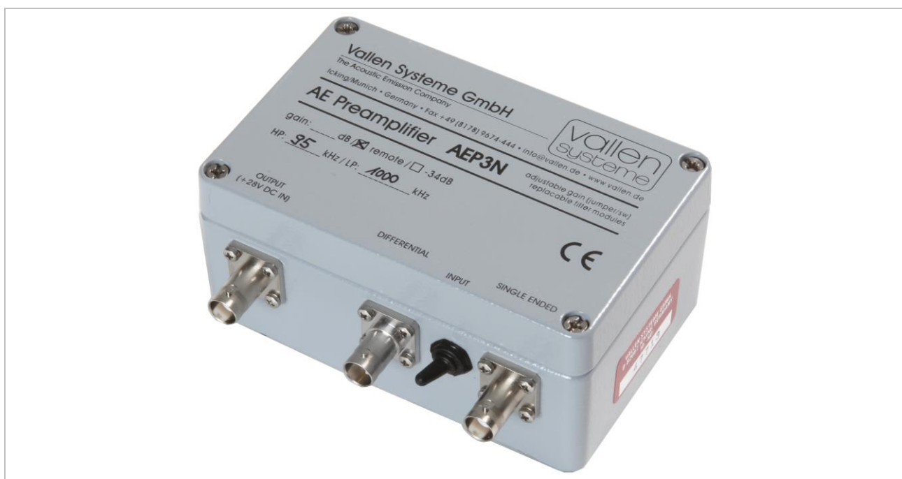
Figure 1: AEP3N preamplifier. Connectors from left to right are: (i) signal output and power supply input, (ii) differential BNO input and (iii) single ended BNC input.
