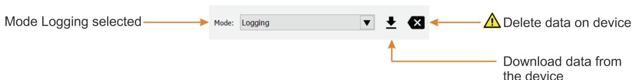
Figure 5: Logging mode with possible actions of downloading data from the device and deleting the data on the device
